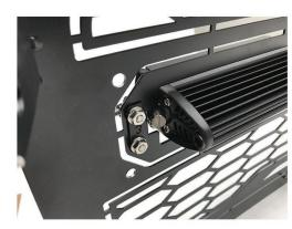
1. Install the supplied trim with hardware. If your installation has ZROADZ LED lights start on one side of each of the (4) openings. Install the trim on the front and the bracket on the back of the grille as shown.
