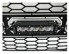
3. Check and secure all hardware. Repeat for remaining light openings.
