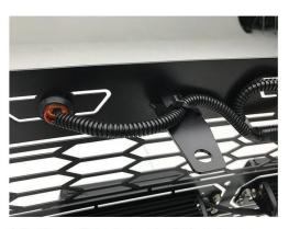
4. Use the supplied amber running light wire harness components to connect each of the (3) lights on top of the grille frame. See harness wire diagram included with components.
