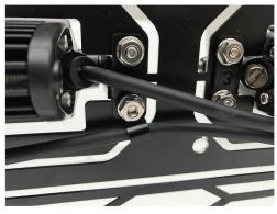
2. If your installation has ZROADZ LED lights use the supplied wire clip on (1) each of the lower side mounting screws as shown to retain the cable.
