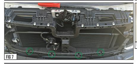
Note the location of the where the Factory Grille is fastened to the vehicle's core support.
