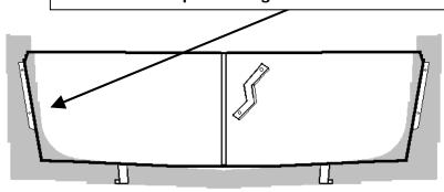
If there is excessive gap between the face of the billet and the grille shell, the lower brackets may need to be adjusted. Bending the brackets will change the position of the grille.
