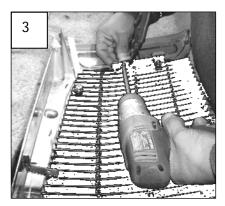
Bend the brackets on the bottom so they sit flat against the bottom of the grille shell (Failure to do this may cause excessive gap between the billet and grille shell).
