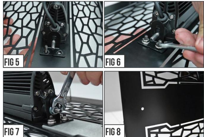
**STEP 3** With LED Light placement set, put into position the remaining bracket and the finally tighten LED and all Mounting Brackets into their final secured position.
