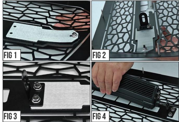
**STEP 2** Put into place one of the Bracket Tabs and secure with provided Hardware as seen in Fig. # 2-4 and then from the backside of grille position LED Light Bar.
