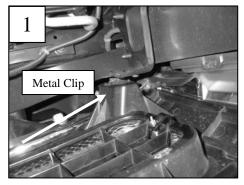
top of the grille. The grille has metal clips along the bottom and center (1); these secure the grille to the core support. Use a slotted screwdriver to release the clips. Remove the grille. If you have purchased the lower grille part #55112; install grills now.
