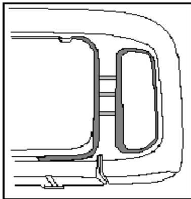
The top of the billet has two dowels that point upwards and three mounting tabs on the bottom. Test fit the billet into the shell. It will be necessary to trim the plastic on each end of the grille shell opening so the billet can sit flush; trim about 1/4" – 1/2" of material off each end. This will allow the billet to sit flush. Trim the three supports molded to the back of the vertical bars on each end.
