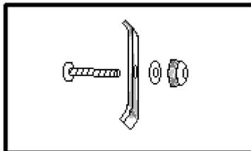
Use the Phillips screwdriver and 5/16" wrench to tighten the hardware. Do not over-tighten; Tighten the insert so it fits snug and even across the shell. Re-install the grille shell assembly back onto the vehicle if needed. ***Thank you for purchasing your T-Rex Billet Grille. 12/14/05***
