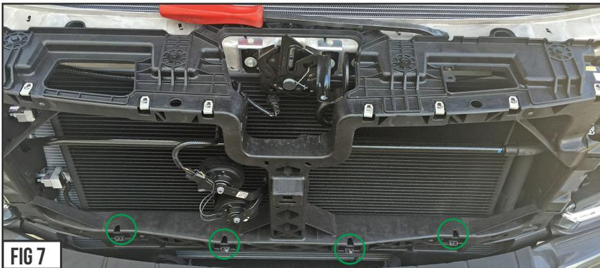
Note the location of the where the Factory Grille is fastened to the vehicle's core support.
