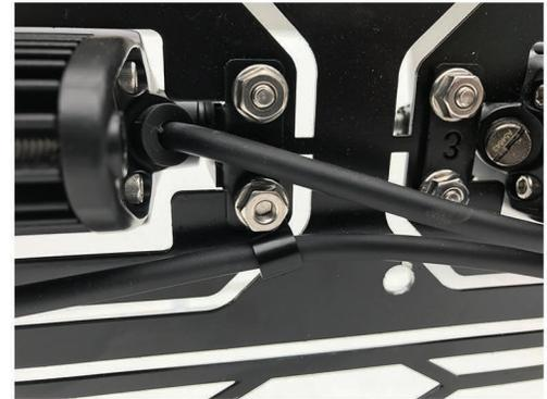
1. Install the supplied trim with hardware. If your installation has ZROADZ LED lights start on one side of each of the (4) openings. Install the trim on the front and the bracket on the back of the grille as shown.
