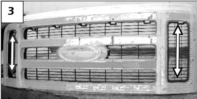
The OE black plastic inserts secured to the side openings (3) must be retained for installation.
