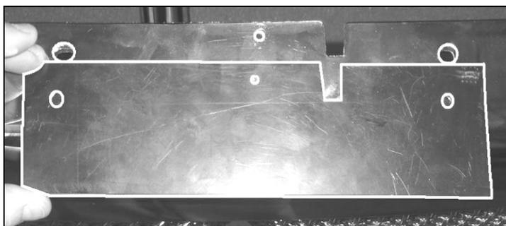
**STEP 6:** Locate the provided template. Place the template on the out side of the grille lined up with the two holes and notch on top of the grille (5). Drill the third hole in the top using this template. Place the last bracket on the inside of the shell. Using the Machine screw and washer, place it through the shell into, the bracket and into the nylon lock nut. Making sure that the mesh lays flat, tighten the hardware.
