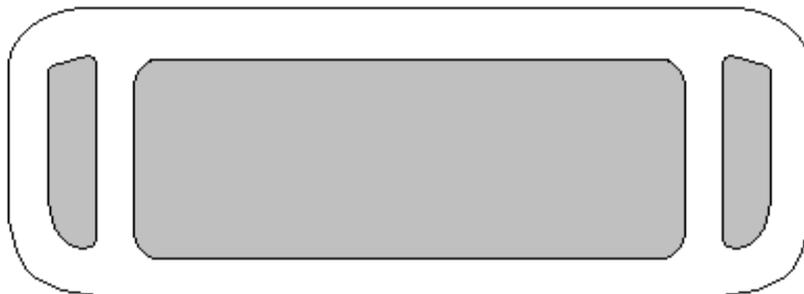
**STEP 4:** Now test fit the mesh in the grille to see if more material will need to be trimmed around the chrome ring. Place the grille face down on a table. Center the mesh in the shell. The mesh should fit flush along the lower and side edges so there is no gap between the mesh and the chrome ring (If it does not, trim the needed areas).
