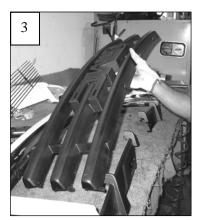
Apply masking tape to the chrome or painted perimeter of the grille. The plastic bar along the top that bolts to the core support must be retained to install the grille. Do not cut this bar from the factory grille. Cut the four vertical bars ½" below the upper cross bar. Now cut the center cross bars from the grille; make three cuts on each end. Make your last four cuts along the bottom. The center bars securing the GMC logo will now separate from the grille (3).
