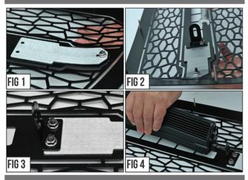
Put into place one of the Bracket Tabs and seucre with provided Hardware as seen in Fig. # 2-4 and then from the backside of grille position LED Light Bar.
