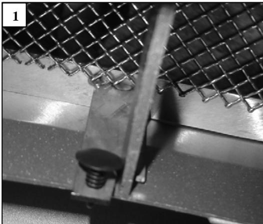
Center the new grille into the bumper opening. From the backside of the bumper; install the push in clips into each bracket (1).
