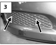
Place a side grille into the correct bumper opening. Mark the grille mounting tabs to the factory insert. Drill a 1/8" hole aligned with each mark (3). Center the grille; insert a screw into each tab. From behind the bumper, secure a #8 flat nut. Tighten hardware and repeat on other side.
