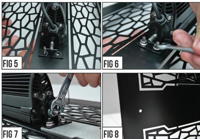
**STEP 3** With LED Light placement set, put into position the remaining bracket and the finally tighten LED and all Mounting Brackets into their final secured position.
