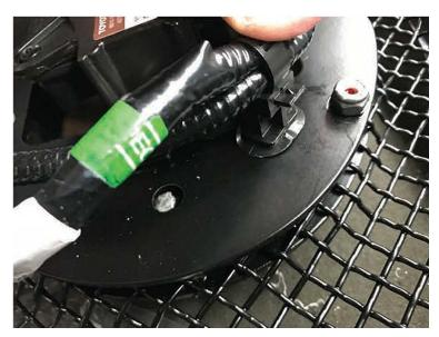
7. Install complete assembly to mounting studs with spacers in place. Use (4) #10 lock nuts and Torque to 30 In-lbs. Note orientation of TOP side of module. Connect ha mess to
