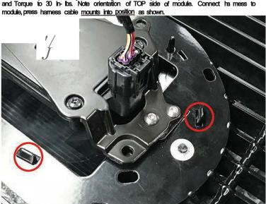
9. Install OEM. front logo as shown. Do not force logo into the logo mounting plate. Insert the lower tabs First, then the upper tabs...
