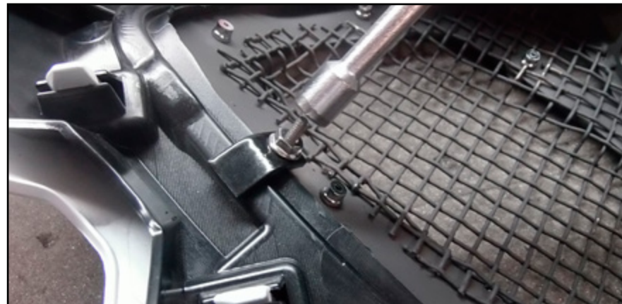
Step 6 Secure grille studs with the included brackets and locknut's.
