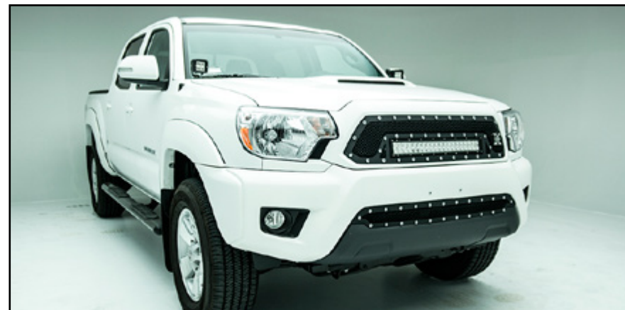
Step 8 Re-install LED light bar into grille. Your installation is now complete. Reattach the grille assembly back to the vehicle in reverse order of removal. Make sure you reconnect and reattach all harnesses, clips and screws. Wire the LED Light Bar via our optional wiring harness kit (part# 639HAR1) or custom wiring harness.
