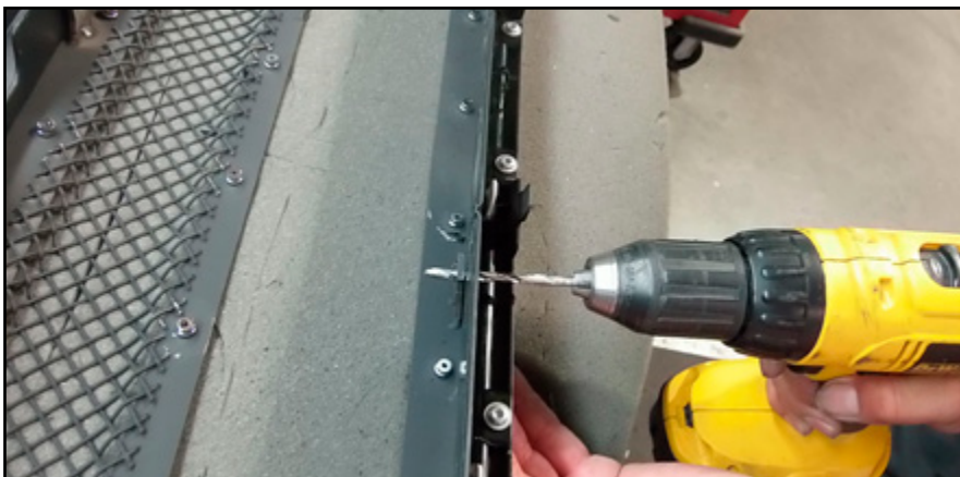
Step 7 Drill 3/16" holes into the grille shell, use the hole on the new grille as a guide. Secure the new grille to the factory grille shell with the supplied screws and flat nuts.
