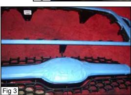
Use a grinding wheel or file to smooth down the areas where you cut out the center section (Fig 4 & 5).
