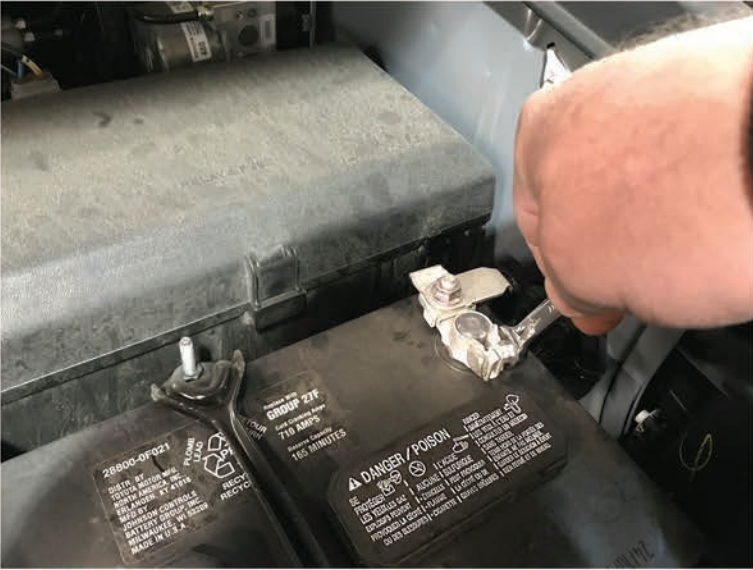
1. Disconnect negative battery terminal.
