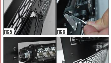
From the face side of grille slip the LED Light bar into place. On the opposite side, position the remaining bracket and finally tighten LED and Brackets into position.
