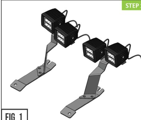
1) The included brackets to not attach directly to the hood, they are installed onto the inner fender panel and extend behind the hood cowl. Once installed they will remain fixed to the inner fender panel, separate from the hood itself.
