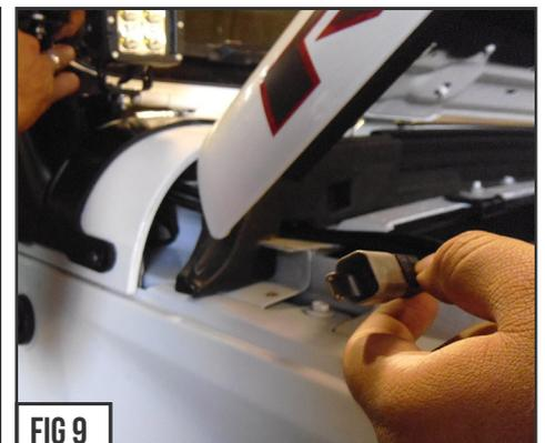
STEP 6 INSTALLERS NOTE: Mock Up LED Lights and plumb wires.
