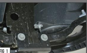
STEP 1 1) From under the rear bumper, take your ZROADZ LED light mount and mock it up into position. This will help you gain familiarity with the mounting orientation. Identify these two bolts that hang the rear bumper on either vehicle corner.
