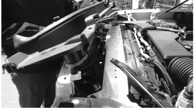
2. Remove the fender flares and pull the front fascia away from the fender on both sides of the vehicle.
