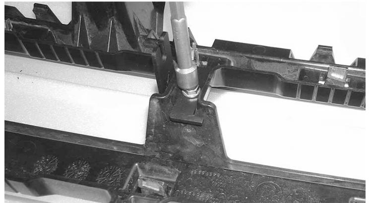
6. Install the LED light to the brackets. Use (1) spacer on each side of the light between the light and the bracket.
