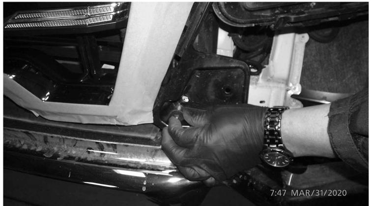
4. Remove the grille from the vehicle and set on a protected work surface.
