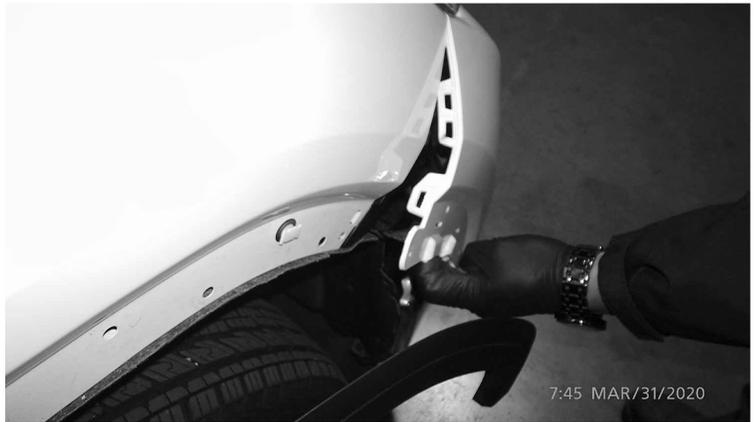
3. Remove the bolts retaining the grille to the core support under the headlight.
