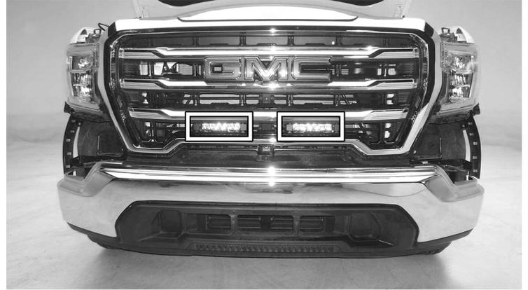
5. From the back side of the OEM grille, install the light brackets and backing plate as shown through the slots in the OEM grille. Use (2) #10-32 flange nuts.
