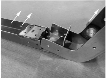
1. Install each leg to the transverse cross member. Use (6) 3/8"x1.00" button head bolts and flange lock nuts for each corner. Do not tighten securely. Make sure holes on the transverse cross member and gate pivot tube are facing the same direction.
