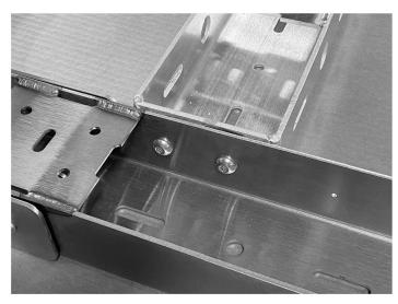
5. Connect the opposite side longitudinal cross bars as shown. Use (2) 3/8"x1.00" button head bolts and flange lock nuts. Torque to 30 ft/lb.
