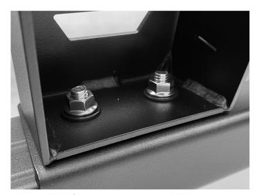
16. Use (2) 3/8" hex lock nuts and (2) flat washers to secure the legs of the rack to the base rails. Tighten the track insert bolts attaching the rail to the bed (From step 14) to secure the rail to the vehicle. Connect the LED lights to the harness, use the supplied wire clamps and push rivets to route the wires along the crossmembers.
