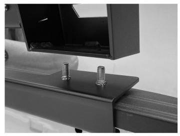
15. Install the assembled rack to the base rails on one side of the vehicle.
