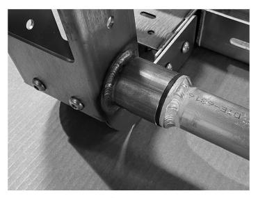
4. Install the gate shaft bushing into the leg housing as shown for both sides of the rack. Install the gate shaft into the bushing. Repeat for opposite side.
