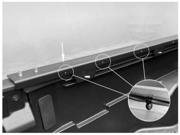
12. Install the driver side base rail as shown above. Run the LED harness along the inside of the base rail. Use the supplied push rivets and wire clamps. There should be approximately 70 inches of the end of the harness extending beyond the hole marked with an arrow.
