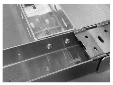
3. Connect one side of both of the longitudinal cross bar as shown. Use (2) 3/8"x1.00" button head bolts and flange lock nuts. Torque to 30 ft/lb.
