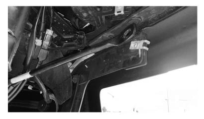
2. Install the bracket using the provided 6mm hex bolt on the outside mounting slot location.
