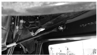
3.On the inside mounting slot use the 6mm hex bolt, washer, lock washer and hex nut.
