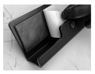
10. Cut (4) pieces of foam and attach adhesive side towards the rail to retain the bolts.
