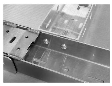
5. Connect the opposite side longitudinal cross bar as shown. Use (2) 3/8"x1.25" button head bolts and flange lock nuts. Torque to 30 ft/lb. Install the harness bracket as shown, use (2) 3/8" flange lock nuts, Torque to 30 ft/lb.
