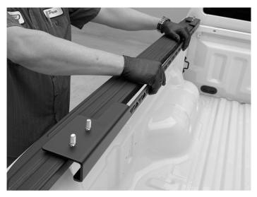
12. Install the driver side base rail as shown. Do not tightnen the clamp bolts under the rail at this time.
