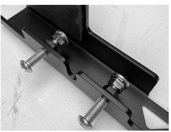
11. Install (8) 2" button cap bolts into each of the (2) rails as shown. Once the thread passes through, install the welded nut with the cap on each bolt. Make sure the bolt is only far enough through to install the nut in order to clear the bed rail of the truck during installation.
