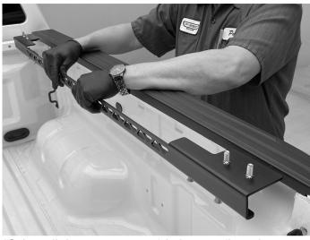
13. Install the passenger side base rail as shown. Do not tighten the clamp bolts under the rail at this time.
