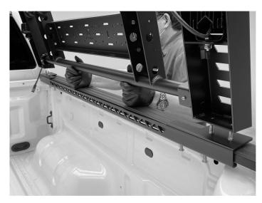
14. Install the rack to the base rails as shown. Center the rack in the bed.
