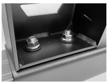
15. Use (2) 3/8" hex lock nuts and (2) flat washers to secure the legs of the rack to the base rails. Secure the clamp bolts under the rail to the bed (From step 11.) to secure the rail to the vehicle.
