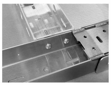
3. Connect one side of both of the longitudinal cross bar as shown. Use (2) 3/8"x1.25" button head bolts and flange lock nuts. Torque to 30 ft/lb.
