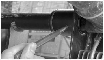
3. Repeat Step #1 on the reverse side of the shaft and mark the center of the locking pin hole.
