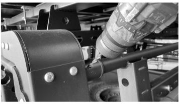
2. Drill a 3/16" pilot hole, then drill a 5/16" final hole as shown.
