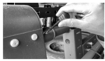
5. Using the provided lock key, unlock the lock assembly and slide the lock pin through the drilled holes.
