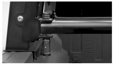
7. To install on the rear gate, replace one side of the lock pins with the lock assembly.
