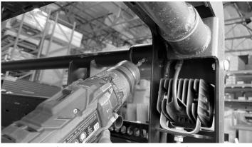
4. Drill a 3/16" pilot hole, then drill a 5/16" final hole as shown.
