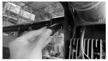
6. Place the lock body onto the lock pin and push the end of the lock in to latch closed.
