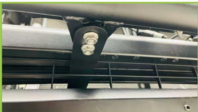
9) Using (2) M8 x 20 MM Bolts and (2) M8 x 1.25 Flange Nuts for each side, secure the (2) lower support brackets onto the bumper top assembly. Tighten all bolts when the bumper top assembly has been leveled and sits firmly.
