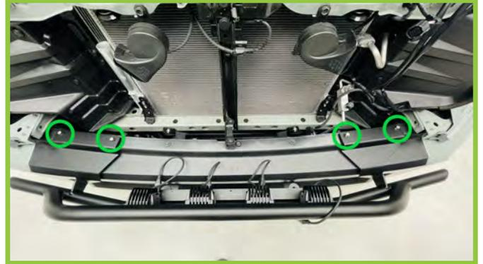
8) Remove the (4) factory bolts circled above. Mount the Front Bumper Top assembly and secure it using (4) M6 x 25 MM Bolts and (4) 1/4" Washers.
