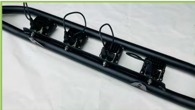
5) Using (1) M8 x 20 Hex Head Bolt, (1) 3/8" x 7/8" Washer, (1) Split Lock Washer and (1) M8 Nut for each LED Pod Light, install each one onto the LED bracket of the assembly.
