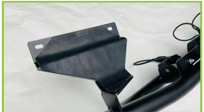
6) Apply the rubber padding onto the underside of the mounting bracket of the assembly. This area will be in contact with the truck's bumper assembly.
