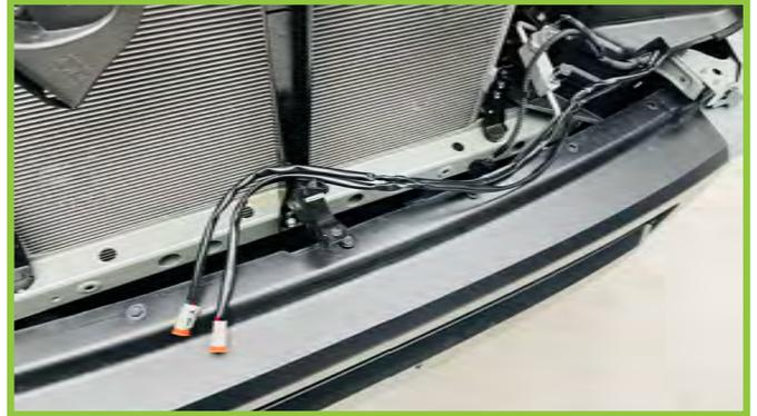
4) If LED pods are to be installed, take this moment to prepare the wiring harnesses for easy plug-in. Use zip ties if necessary.
