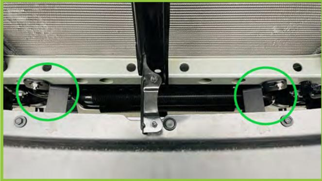
7) Install the lower support brackets as shown above. Using (1) M8 x 20 MM Bolt that extrudes from the inside, secure each bracket with (1) Washer and (1) M8 x 1.25 MM Nut for each bracket. Lightly tighten for now to leave room for adjustment later.
