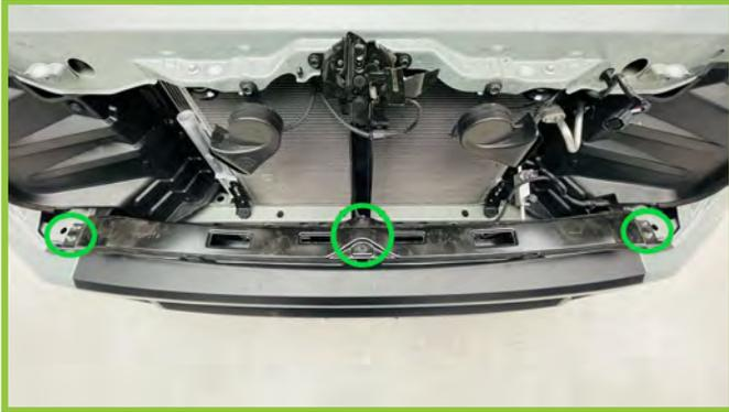
3) Remove the following cover by removing the (6) flange nuts as indicated above.
