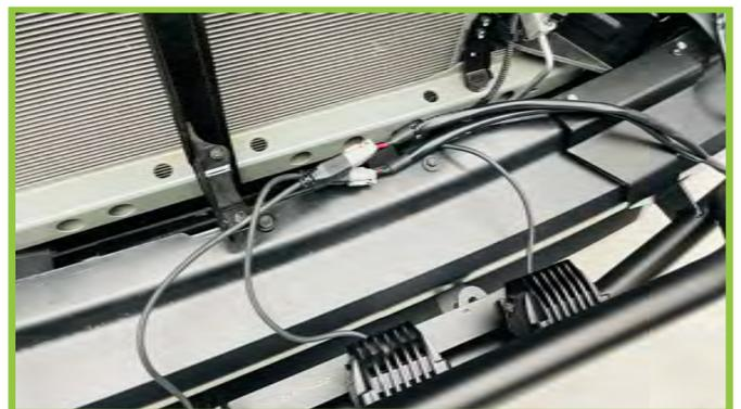
10) Plug-in the LED Pods to their respective harness and check for functioning light. Re-install the covers, brackets and grille. This concludes the instruction guide for Z329661.
